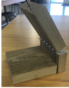
Figure 3A: Built the foam testing ice bag press without the velcro or foam attached
