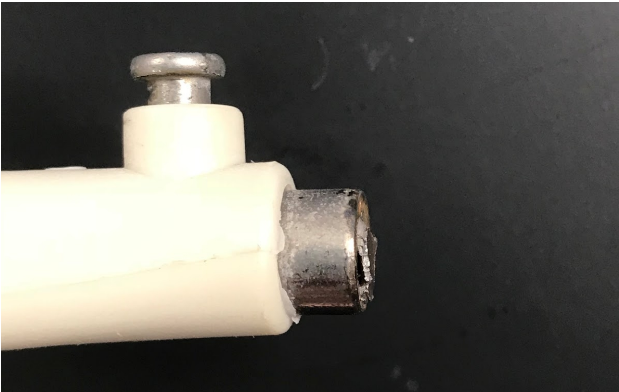
Figure 11: This is a side profile image of the weld that connected the bowl to the handle of the ice cream scoop.
