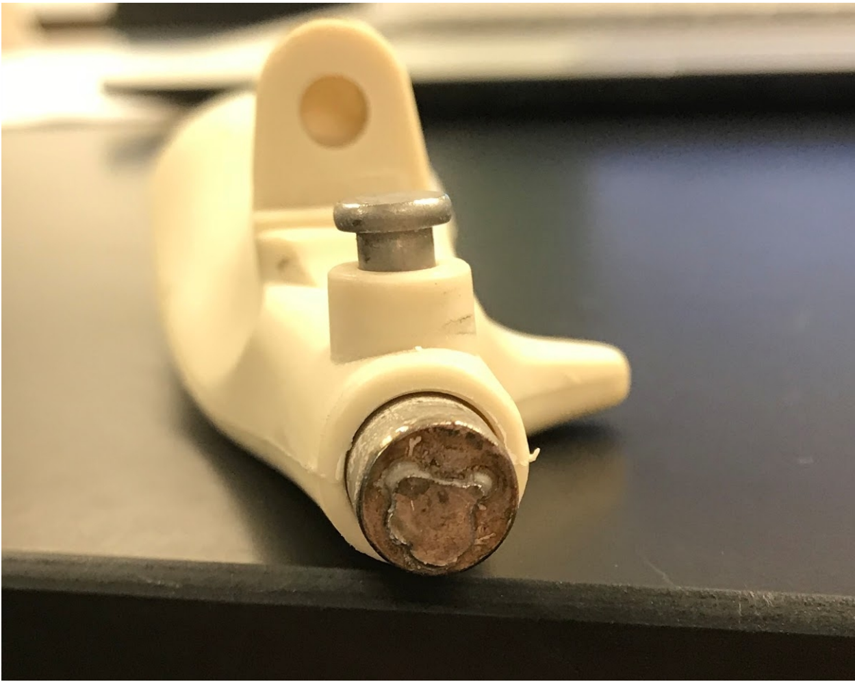
Figure 10: This picture is an image of the handle and shows the size of the weld relative to the size of the handle of the ice cream scoop.
