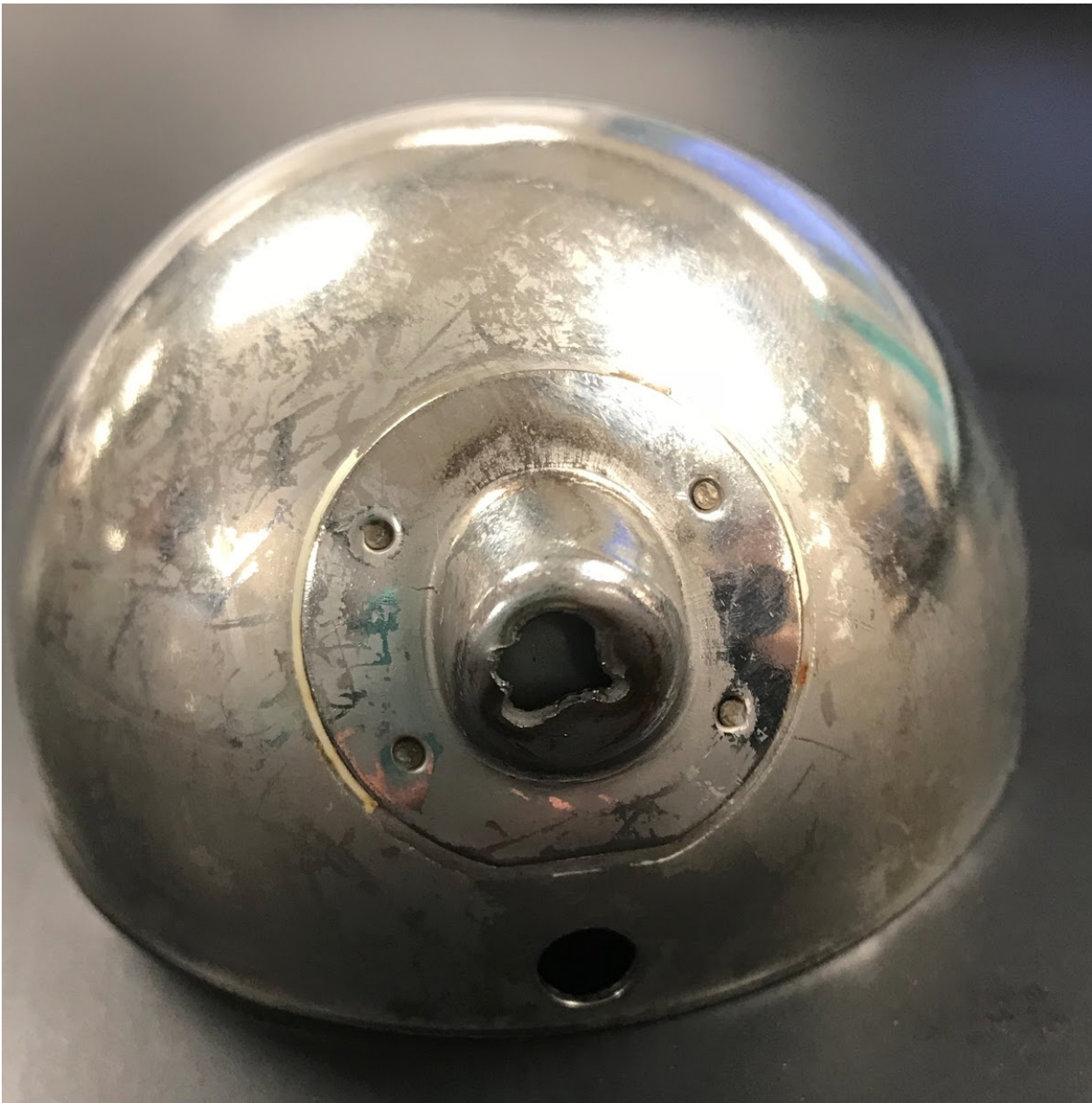
Figure 9: This is an image of the ice cream scoop's bowl that broke off of the handle.
