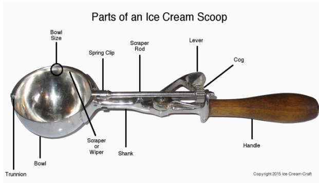
Figure 1: Diagram labeling the parts of an ice cream scooper similar to the type being analyzed. Taken from icecreamcraft.com
